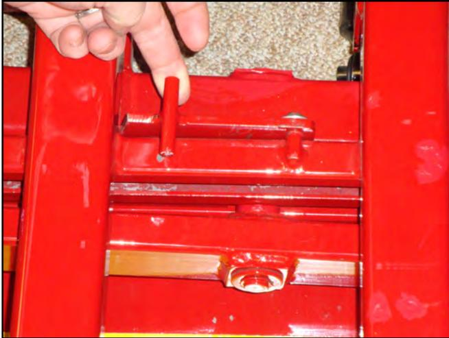
5. While holding both latches up and lift the top frame pass the latches until it is at its full, upper most position. Have the assistant hold the weight and insert the pivot pin in the hole in the base frame. See Fig. 8. With the PalletPal in this full upper most position the orange spring can be installed.
