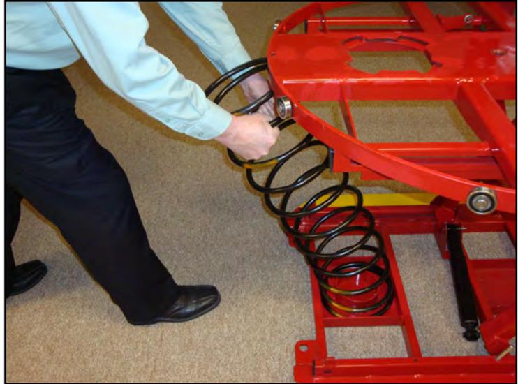
7. Grasp the spring by the second or third coil down from the top (do **NOT** grasp the top coil or rung) and push the spring down and under the edge of the top frame.
