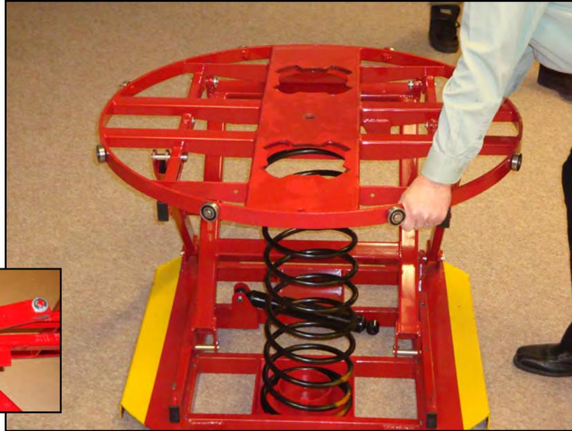
9. Remove the shock absorber pivot pin. Push down on top frame until latches engage. (Both latches will drop into place).
