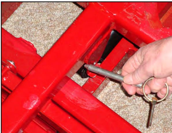
3. The shock absorber is attached to the top frame of the unit with a pivot pin, and this is held in place by a linch pin. The pivot pint is used to hold the table frame in the raised position. Take a look at the mechanism and note the positions of the parts. Remove the linch pin and remove the pivot pin. Lay the free end of the shock absorber down.
