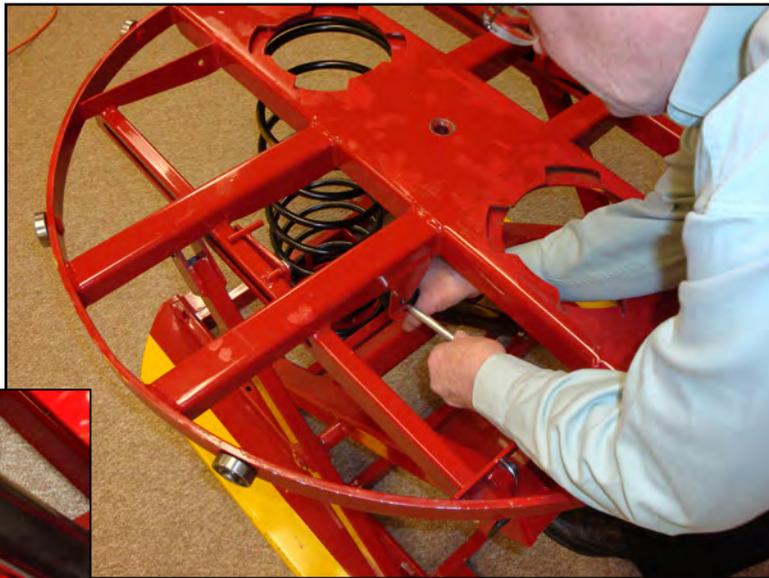
10. Reinstall the shock absorber pivot pin and linch pin.
