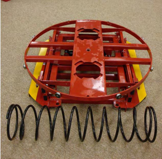
2. The unit is shipped without springs installed. The installation of the first spring (orange) requires two people. Lift off rotating ring and both yellow bayonets. Set them aside, they will be installed later.
