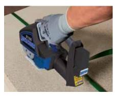
The B1000 can pull up to 1125lbs of tension and operate with both polypropylene and polyester plastic strapping, 5/8" to 3/4" wide, .031-.050" thick. No special change parts are
