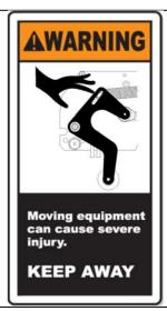
The label shown is affixed to the top squeezer assembly brackets on either side of the machine. They warn the operator of a potential pinch point between the top of the case and the top squeezer rollers. Keep hand away from this area when processing a case
