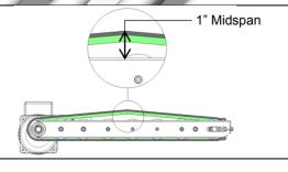
After Tensioning, The Belt Must Be Properly tracked In Idler Pulley To Be Sure That The Tracking bead Is Properly centered in the idler pulley groove.
