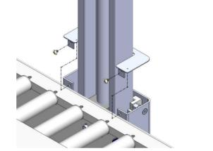
Using A 3 Mm Allen Key, A 10 Mm Wrench And A 12 Mm Wrench, Adjust Upper Column Guide Bolts To Reduce Clearance Between Column And Guide.
