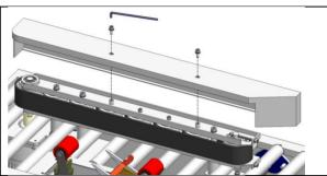
Using a 4 mm Allen Key and 10 mm Wrench, Loosen Upper and Lower Belt Tensioning Bolts.
