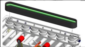
Using a 4 mm Allen Key and 10 mm Wrench, Tighten Upper and Lower Belt Tensioning Bolts.
