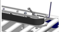
Proper Belt Tension Is Achieved When A 5 Pound Pull Force Is Used To Create A 1" Gap As Shown In The Middle Of The Drive Base.
