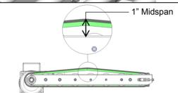
After Tensioning, The Belt Must Be Properly tracked In Idler Pulley To Be Sure That The Tracking bead Is Properly centered in the idler pulley groove.
