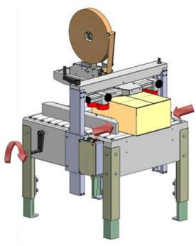
Until Side Drive Belts Contact Case. Side Drive Belts Should Contact The Case Firmly Enough So Case Processes Smoothly But Not So Firm As To Score The Side Of The Case.
