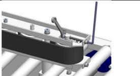
Proper Belt Tension Is Achieved When A 5 Pound Pull Force Is Used To Create A 1" Gap As Shown In The Middle Of The Drive Base.
