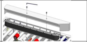
Using a 4 mm Allen Key and 10 mm Wrench, Tighten Upper and Lower Belt Tensioning Bolts.
