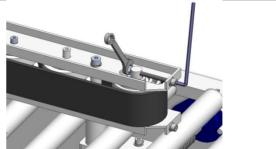
Remove Worn Belt And Replace With New Belt
