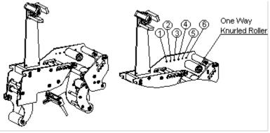
Move the guiding tape wheel from hole #1 to hole #6 to shorten the tape length.
