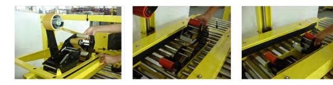
Check tape cutter position and adjust as needed.
