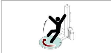
Danger of collision and slipping: do not come near machineparts during its operation.
